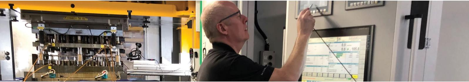
Precision lubrication system for **stamping, pressing and punching processes** which reduces the oil consumption with more than 40% and saves water and liquids in the subsequent cleaning process of machined parts.
